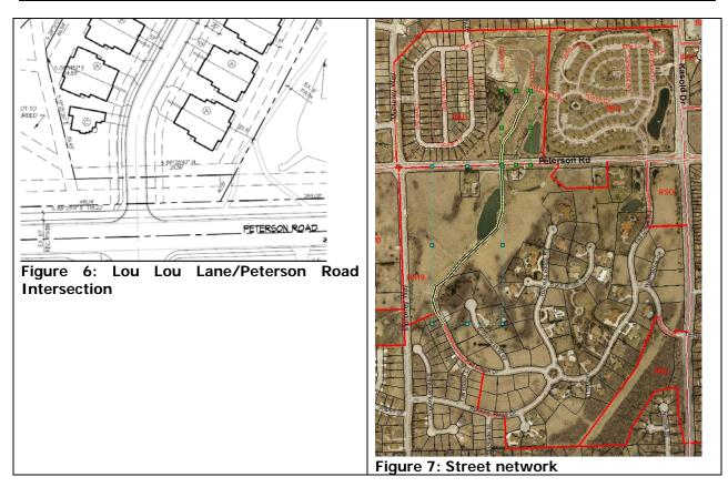
**Street Design:** The interior street network is proposed as a private street configuration. The Preliminary Development Plan is conditioned to provide a standard 27' street cross section. The plan currently shows sidewalks on only one side of the private street. Note 1.9 must be revised to also note the street width shall be 27'.
