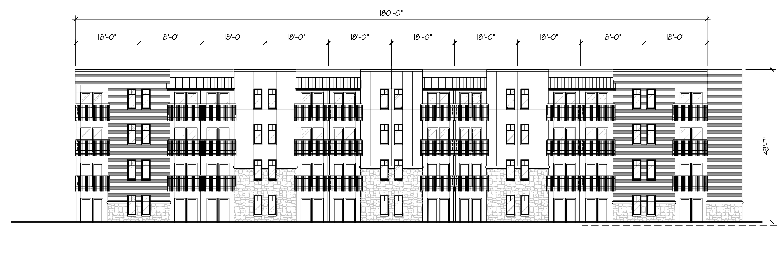
INDEPENDENT LIVING BUILDING NORTH ELEVATION SCALE: 1/16" = 1'- 0"
