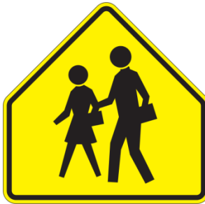
Figure 1. School Zone Sign (S1-1)
