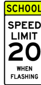
Figure 4. School Speed Limit (S5-1)
