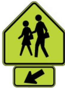
Figure 6. School Crossing Assembly (School S1-1 with Diagonal Downward Arrow W16-7P)
