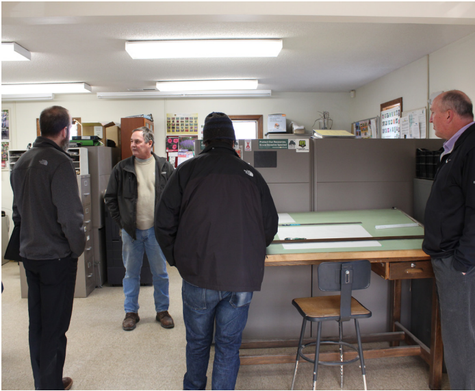
Linoleum flooring, painted gypsum board walls, popcorn ceiling, surface mounted fixtures
