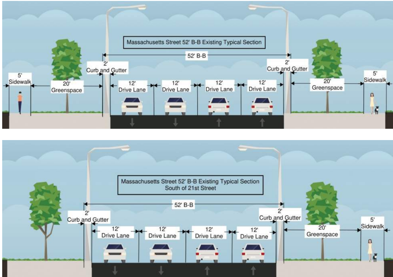
Figure 2 – Existing Typical Section
